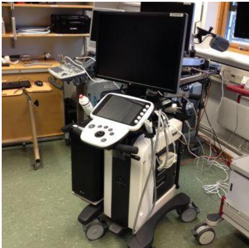
**The Regional Anaesthesia Assistant (RAAs) is composed of a high-tech ultrasound system, magnetic probe tracking, additional computer hardware, and a large screen to display the augmented reality**
