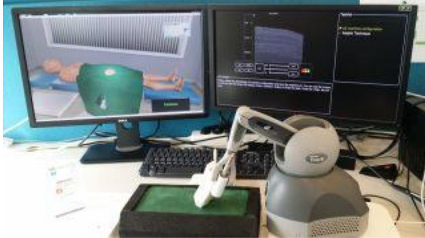
**The Regional Anaesthesia Simulator (RASim) prototype shows a haptic device with the needle on a foam rest. Two screens are required for the situs (left) and the courseware (right).**
